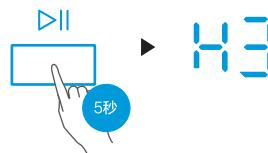
3 按启动/暂停键
