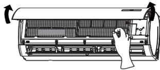
从空气滤尘网上取下冷触媒过滤网
