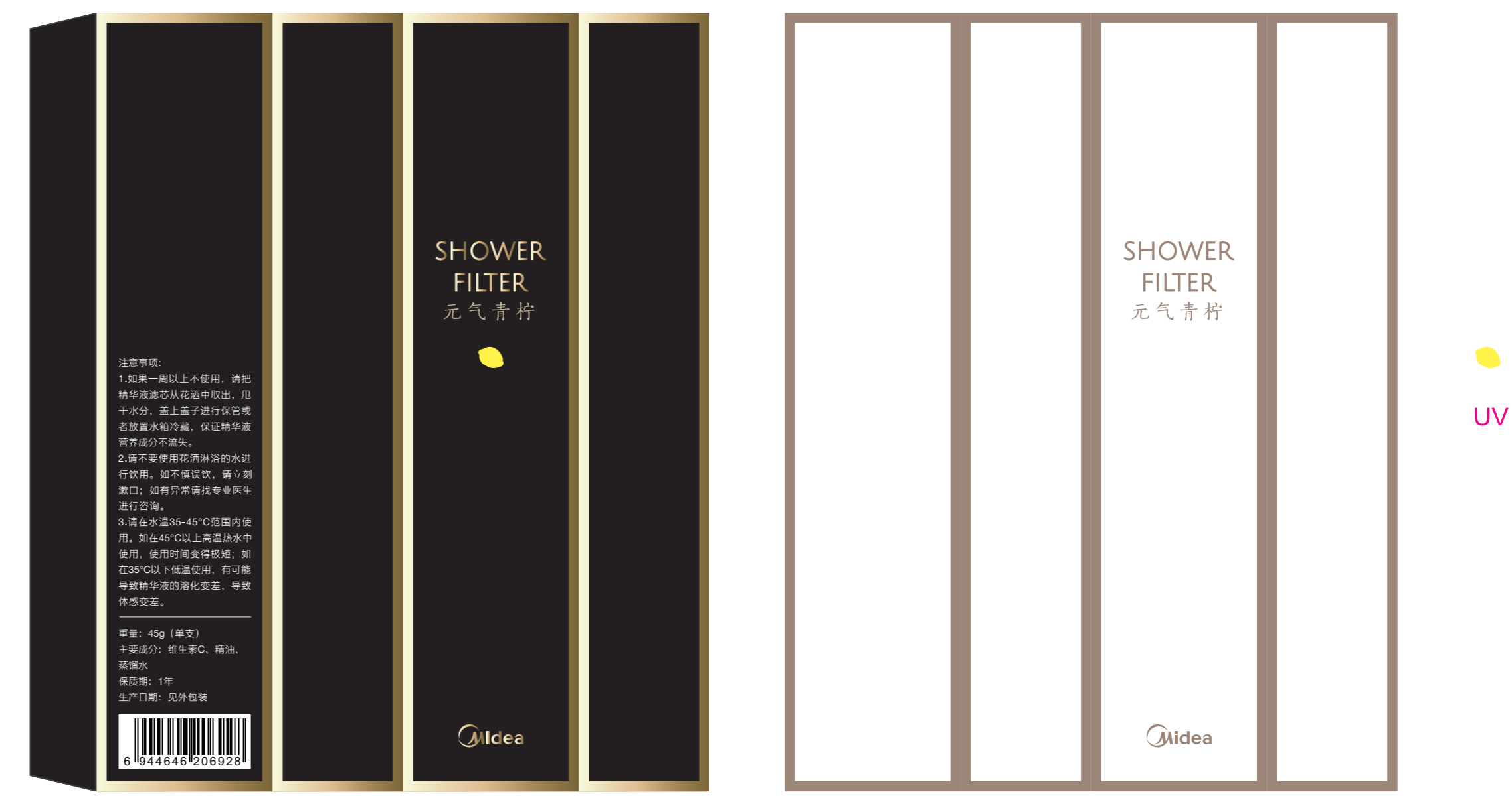
美的S002滤芯(1芯)抽屉盒 材质: 400g单粉, 烫金+UV, 尺寸: 35x26x155mm, 尺寸公差±2mm 烫金10154C+UV专色1-7C
